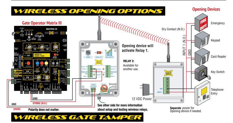
The **GATE TAMPER** can be used for various functions such as turning a warning light, siren or camera on when the gate is tampered with (Vandalized Gate). The gate operator defines a "Vandalized Gate" as **UNAUTHORIZED** movement of the gate. This can occur if the chain is dropped and gate is manually moved from the **closed position** or the gate is forced open from the **closed position** without authorization.
