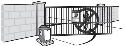
6. The gate must be installed in a location so that enough clearance is supplied between the gate and adjacent structures when opening and closing to reduce the risk of entrapment. Swinging gates shall not open into public access areas.
