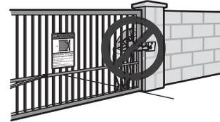
9. The Stop and/or Reset (if provided separately) must be located in the line-of-sight of the gate. Activation of the reset control shall not cause the operator to start.
