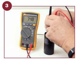
Using a multi-meter, measure the capacitance between the capacitor contacts. The measurement on the meter should be within 10% of the uF rating on the label.
