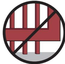
Gate MUST have a smooth bottom edge, no protrusions should exist.
