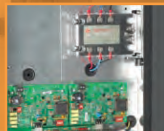
Solid State Motor Control no relay contacts to wear out or burn
