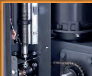
Limit Switches direct driven and easily adjustable
