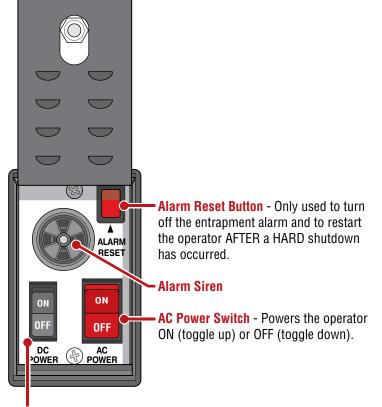
**DC Power Switch** - Turns the DC system power ON (toggle up) or OFF (toggle down).
