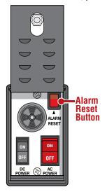
• Before resetting a hard shutdown, determine why the shutdown occurred. Inspect the gate for any obstructions along its path that could have activated the inherent entrapment sensing system. Inspect the gate and gate hardware.
