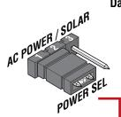
Important: Pins 1 and 2 **MUST** be jumpered together when using AC input power.
