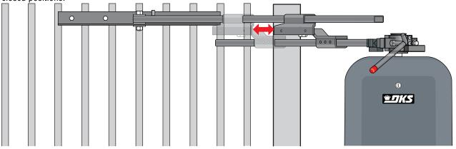
Mark and cut off excess arms. Secure arms to elbow assembly with 6 allen screws. Tighten hub and replace release tool. Install safety covers.
