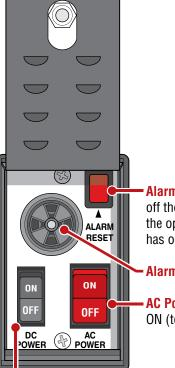
Alarm Reset Button - Only used to turn off the entrapment alarm and to restart the operator AFTER a HARD shutdown has occurred.
