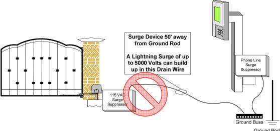
For Best Results, locate the Surge Suppression Devices <u>at the Ground Rod</u>, then run to the equipment you are protecting!
