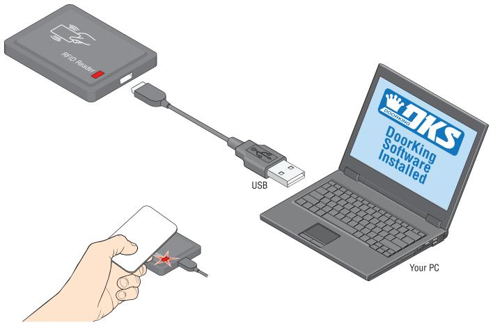
Place the card on the card scanner to read card code. LED will flash.
