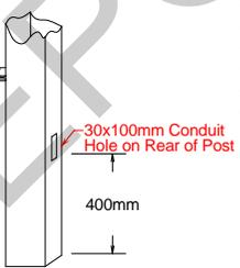
← 30 x 100 mm Conduit Hole on Rear of Post
