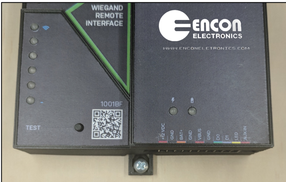
Figure 7: Bottom DIN Rail Screw Mount
