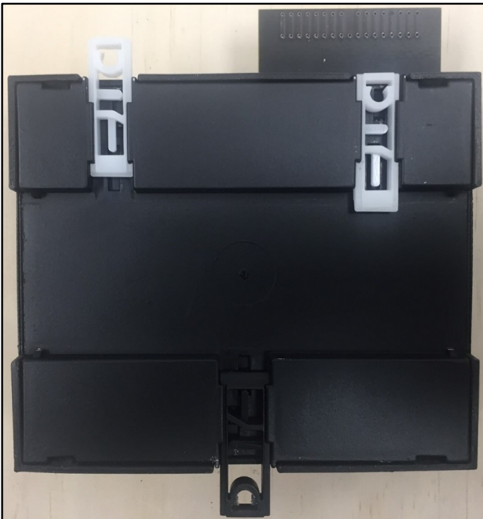
Figure 5: DIN Rail Mounting Pins
