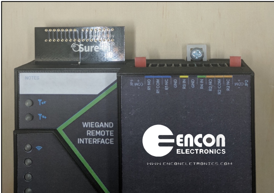
Figure 6: Top DIN Rail Screw Mount
