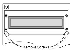
Install the heater assembly with the nylon washers supplied. The nylon washers MUST be installed between the heater assembly and the display circuit board. Replace the screws removed in step 1.
