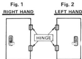
Left-Hand Doors – From exterior of door, hinges are on left-side. (Fig. 2)
