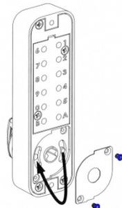
Now, move the pin from the right side of the outside body to the hole on the left side. Replace plate and screws.
