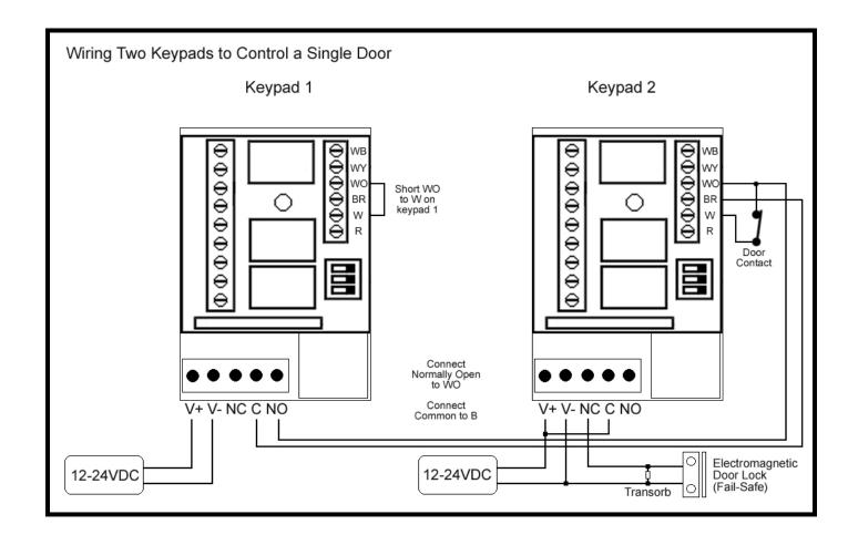
The diagram above shows how to connect two keypads to control a single door. Entering your code on keypad 2 unlocks the maglock directly. When you enter your code on keypad 1, it triggers the REX input of keypad 2, which unlocks the door.
