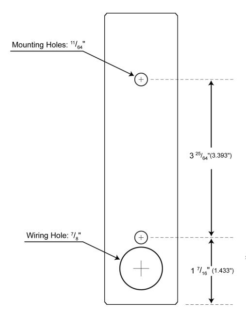
The iLM keypad is designed for surface mount applications. You must drill a <sup>7</sup>/<sub>8</sub>" hole for the wire harness connector as shown so the unit is flat against the mounting surface.
