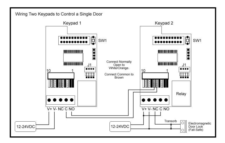
The diagram above shows how to connect two keypads to control a single door. Entering your code on keypad 2 unlocks the maglock directly. When you enter your code on keypad 1, it triggers the REX input of keypad two, which unlocks the door
